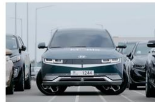
Hyundai vehicle demonstrating “crab walk” manoeuvre. Source: Hyundai Mobis
